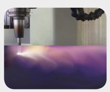
Photo A shows a conventional tool dry cutting a carbon fibre component. Without the use of air or flood coolants the cutter becomes extremely hot. The jet of dust particles created by the cutter is super-heated and can damage the surface of the carbon fibre component.
